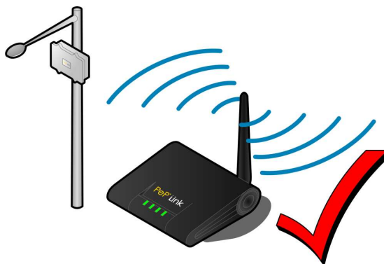
Figure 4 – Orienting the antenna vertically allows signals to span out.
