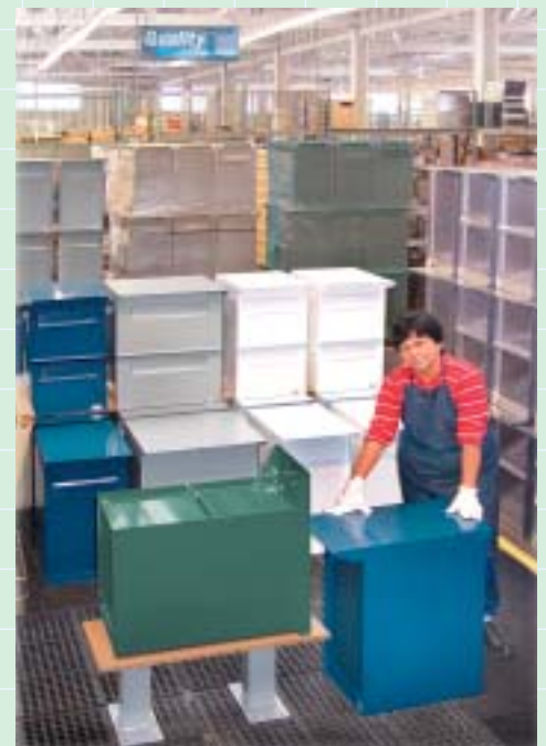
Final inspection of pedestal drop boxes
